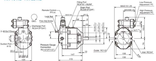
Note: - Inlet - Outlet port are for standard rotation (clockwise)
