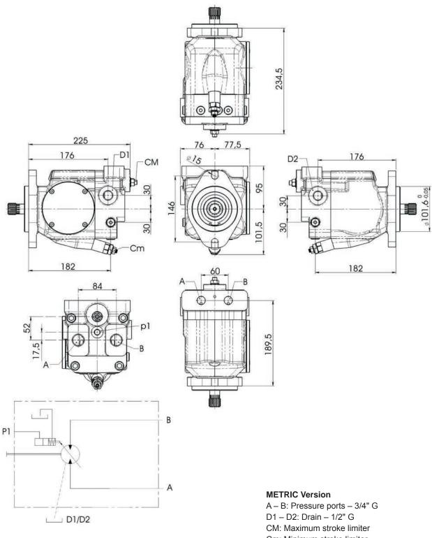
Cm: Minimum stroke limiter P1: Pilote pressure -1/4" G
